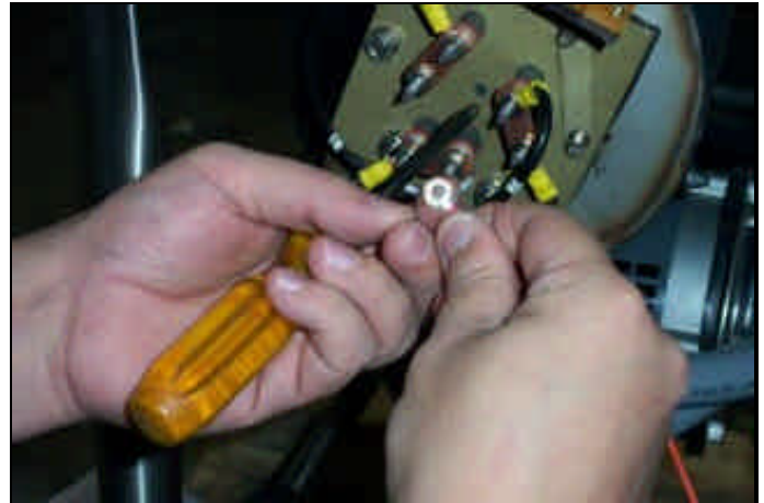
Fitting the jumper into the mounting cup.
